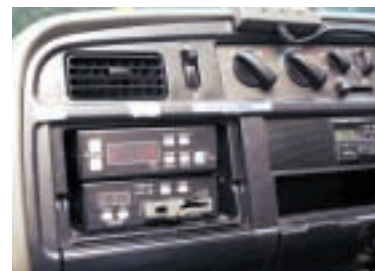
Thermometer mounted in a delivery truck
