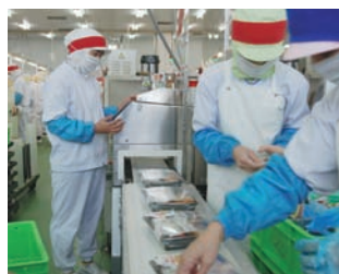
Metal detector checks for foreign substances
