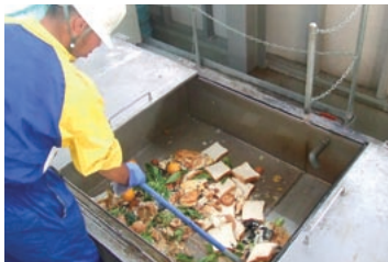
3. Leftover food put into a liquefier and then fermented
