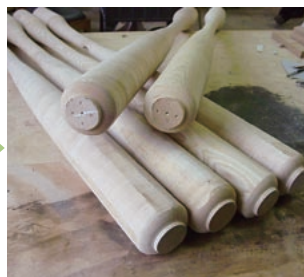
Around 4 to 10 bats can be produced from 1 tree and approximately 10% of the wood is unsuitable for bats.
