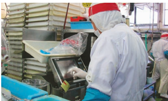
Weighing of raw materials at rice production facility reduces waste.
